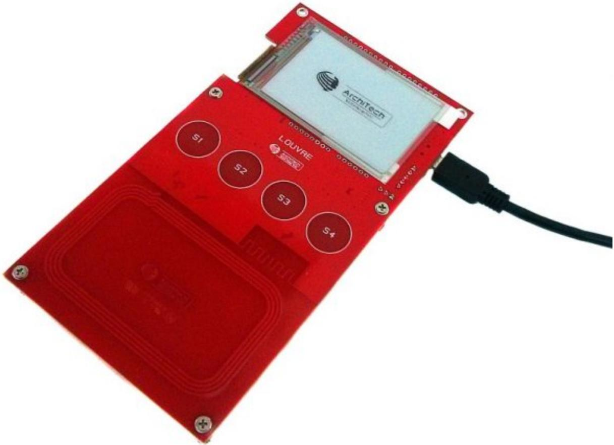
3. The Louvre display on the e-paper screen the temperature read from **SE98ATP** sensor and the last capacitive button pressed.
