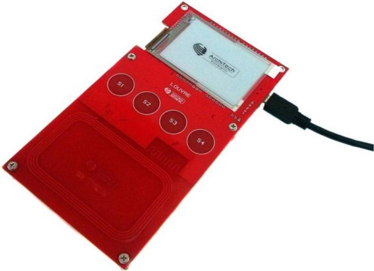
3. The PC will see the Louvre board as a storage memory, delete the old **firmware.bin** file and copy the newer **firmware.bin** file into the mass storage.
